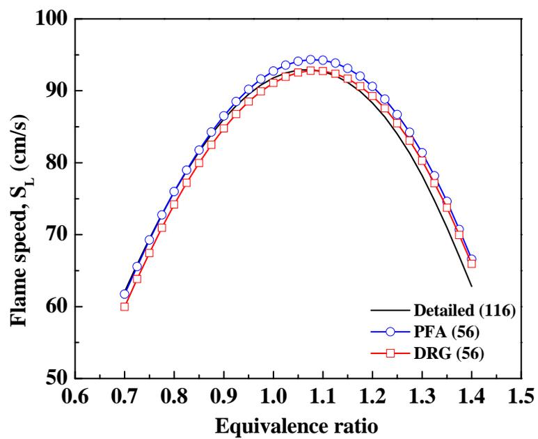
Fig. 9 The laminar flame speed as a function of equivalence ratio for n-heptane/air mixtures at 500 K and 1 atm.
