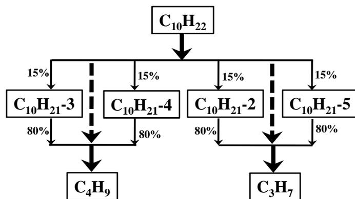
Fig. 6 Homogeneous ignition reaction path of n-decane at  $P=1$  atm,  $\tau=4.67 \times 10^{-5}$  s,  $T=1197$  K,  $\Phi=1$
