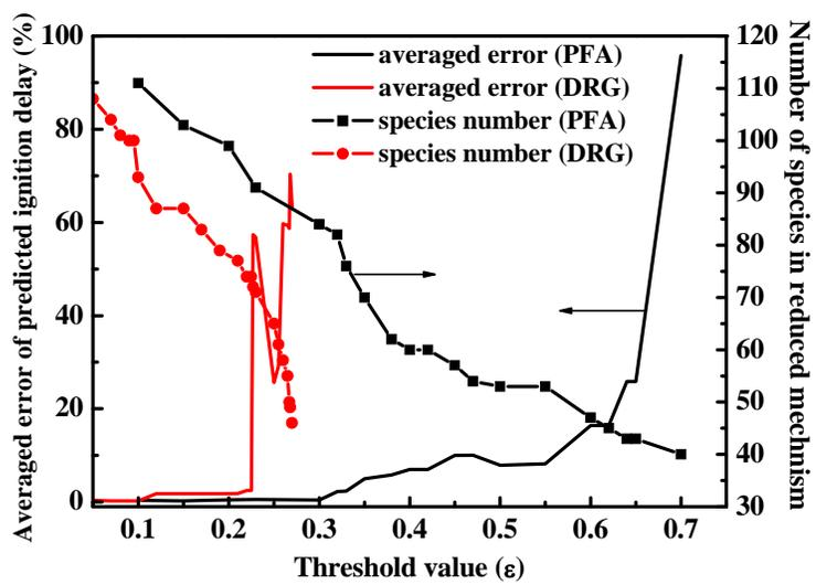
Fig. 14 Averaged error of ignition delay predicted by reduced mechanisms and the number of species in the reduced mechanism as a function of the threshold value for a stoichiometric n-decane/air mixture at 1 atm
