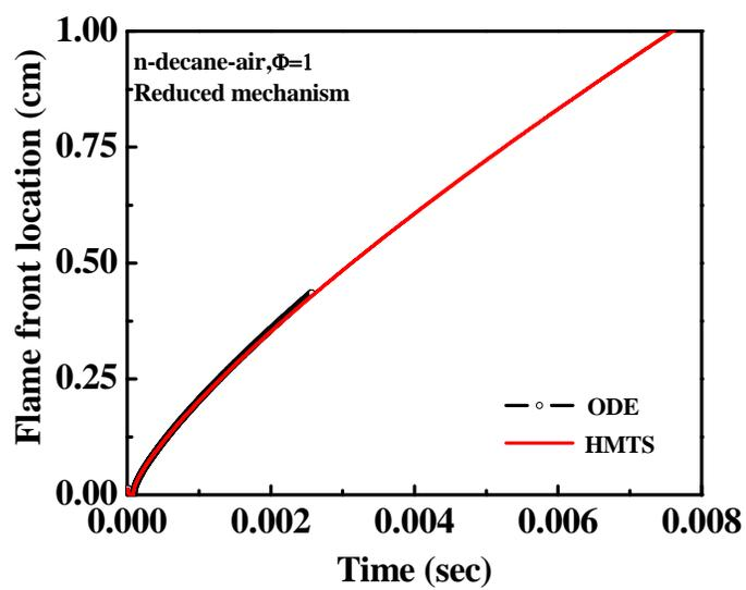
Fig. 17 Flame front location as a function of time for propagating spherical n-decane/air flames by ODE and HMTS methods
