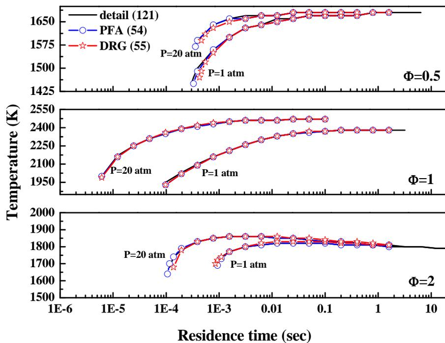
Fig. 3 Comparison of PSR-simulations of lean, stoichiometric, and rich n-decane-air mixtures for various temperatures and pressures predicted by using reduced mechanisms generated by PFA and DRG as well as detailed mechanism
