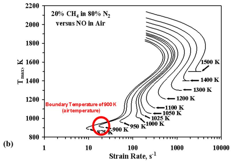
Fig. 7 (a) Ignition pathway of CH<sub>4</sub> at the highest temperature point, (b) S-curve response for 12% CH<sub>4</sub> in N<sub>2</sub> vs preheated air with 10,000 ppm NO as a function of maximum temperature and strain rate
