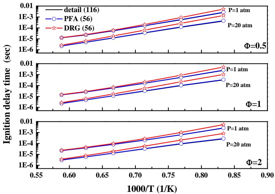
Fig. 4 Comparison of ignition delay times of lean, stoichiometric, and rich n-heptane-air mixtures for various temperatures and pressures predicted by using reduced mechanisms generated by PFA and DRG as well as detailed mechanism
