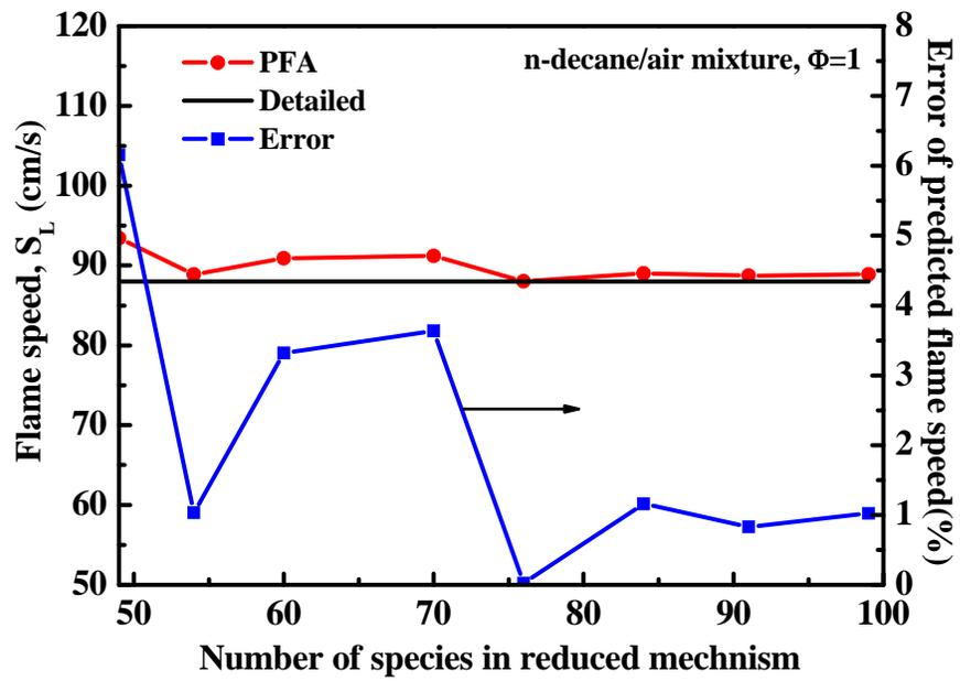
Fig. 16 The laminar flame speed and the error predicted by the reduced mechanism as a function of number of species in reduced mechanism for a stoichiometric n-decane/air mixture at 500 K and 1 atm
